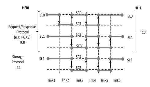
FM allocates and configures TCs, SLs, SCs and VLs based on sysadmin vFabric input
