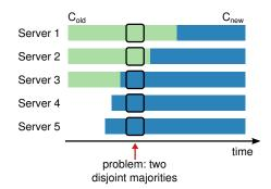
**Figure 8:** Switching directly from one configuration to another is unsafe because different servers will switch at different times. In this example, the cluster grows from three servers to five. Unfortunately, there is a point in time where two different leaders can be elected simultaneously, one with a majority of the old configuration ( $C_{old}$ ) and another with a majority of the new configuration ( $C_{new}$ ).
