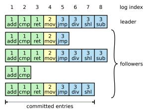
**Figure 5:** Logs are composed of entries, which are numbered sequentially. Each entry contains the term in which it was created (the number in each box) and a command for the state machine. An entry is considered *committed* if it is safe for that entry to be applied to state machines.
