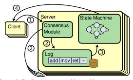
Figure 1: Replicated state machine architecture. A consensus module manages a replicated log containing state machine commands from clients. The state machines process identical sequences of commands from the logs, so they produce the same outputs.
