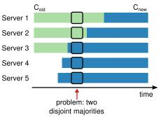
**Figure 10:** Switching directly from one configuration to another is unsafe because different servers will switch at different times. In this example, the cluster grows from three servers to five. Unfortunately, there is a point in time where two different leaders can be elected for the same term, one with a majority of the old configuration  $(C_{old})$  and another with a majority of the new configuration  $(C_{new})$ .
