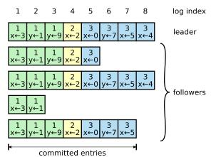
**Figure 6:** Logs are composed of entries, which are numbered sequentially. Each entry contains the term in which it was created (the number in each box) and a command for the state machine. An entry is considered *committed* if it is safe for that entry to be applied to state machines.
