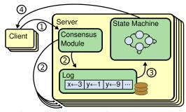
**Figure 1:** Replicated state machine architecture. The consensus algorithm manages a replicated log containing state machine commands from clients. The state machines process identical sequences of commands from the logs, so they produce the same outputs.
