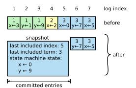
Figure 12: A server replaces the committed entries in its log (indexes 1 through 5) with a new snapshot, which stores just the current state (variables x and y in this example). The snapshot's last included index and term position the snapshot in the log preceding entry 6.
